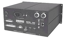
The Model 1200 concurrently processes the video from two Newton Labs Line Scan Cameras where simultaneous inspection from both cameras is required. It is commonly used to increase the number of pixels (and thus the resolution) when the resolution from a single line scan camera is not sufficient for the application or to perform two different inspections simultaneously (such as the top and bottom of the same web).
