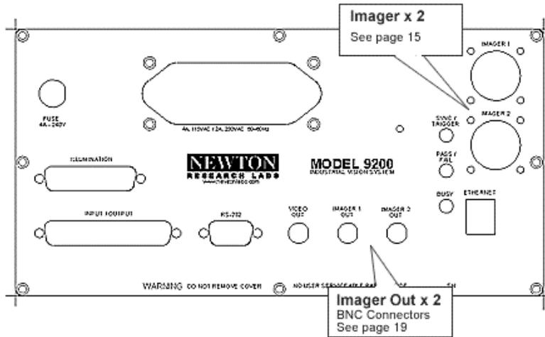
Figure 3. Model 9200 Front Panel
