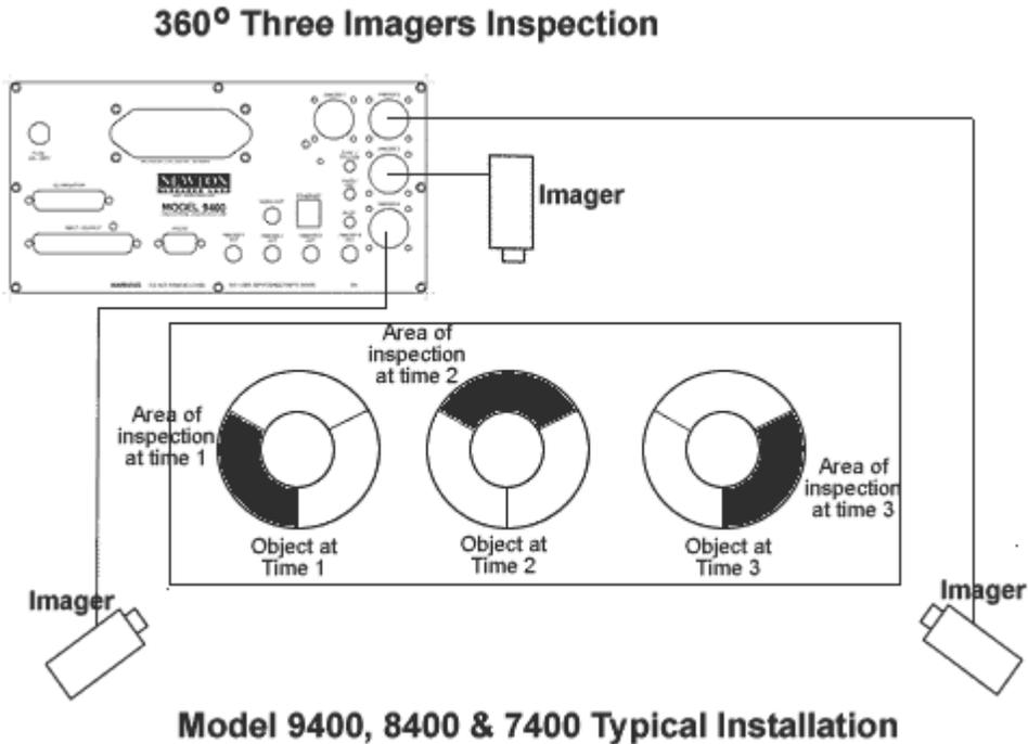
**Figure 10. Model 9400 Typical Installation--360° Inspection**
