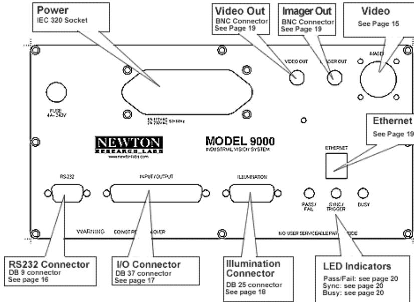
**Figure 2. Model 9000 Front Panel**
