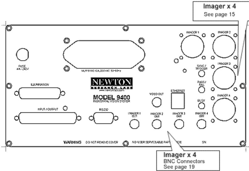
Figure 4. Model 9400 Front Panel
