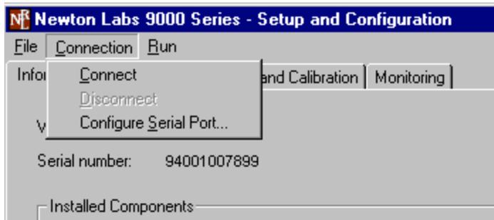
**Connect**—Connects the Newton Labs Software Component User Interface to a Newton Labs Vision System. *This option must be selected first in any setup session.*
