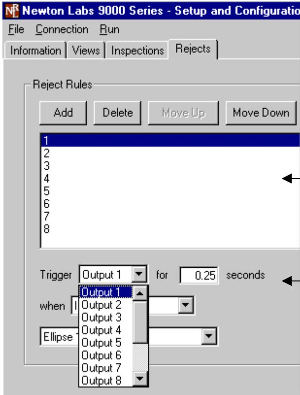
Establish a new reject rule by clicking “Add”, or select an existing reject rule from the list in the window.
