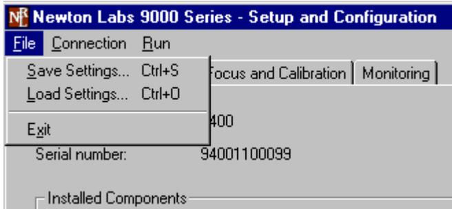
**Save Settings**—Saves currently selected settings to a file on the laptop or PC you are using. A dialog box will ask for a file name and location. It is highly recommended that you save the settings after a successful setup.
